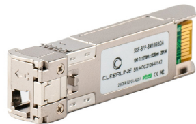
SSF-SFP-SM10GBDA 10G SFP+ transceiver BiDi T:1270/R:1330nm, 20Km max
