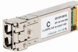
SSF-SFP-SM10G 10G SFP+ transceiver SM, 1310nm, 20Km max reach
