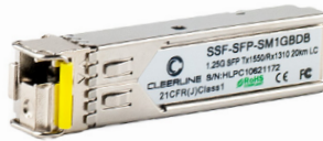
SSF-SFP-SM1GBDB 1G SFP transceiver BiDi T:1550/R:1310nm, 20Km max reach
